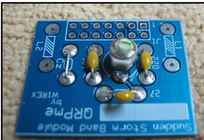
Band module board with caps installed.
